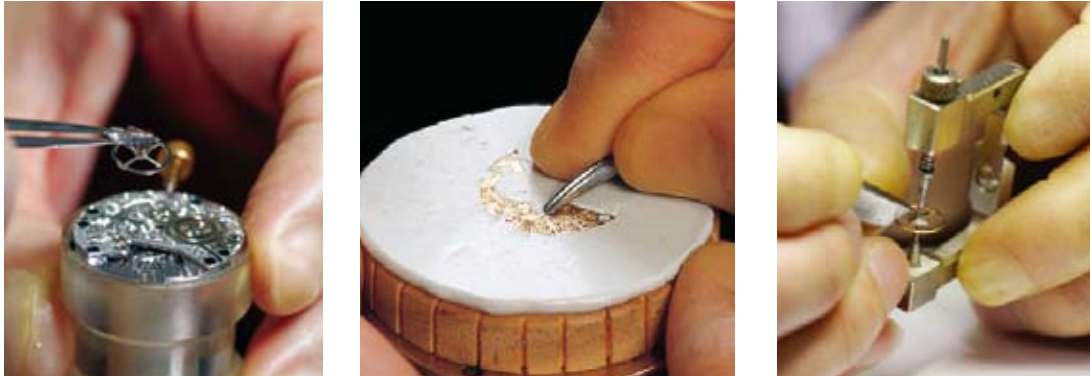
Mamoru Sakurada mounting the balance into the 1.98mm Credor movement. (left) Kiyoshi Terui engraves a Credor watch in his own style, and using tools he himself created. (center) Akira Ohira adjusts the balance of each and every Grand Seiko movement. (right)
