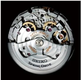
The clearly visible glide wheel turns exactly 8 times per second, regulating the movement of the hands.
